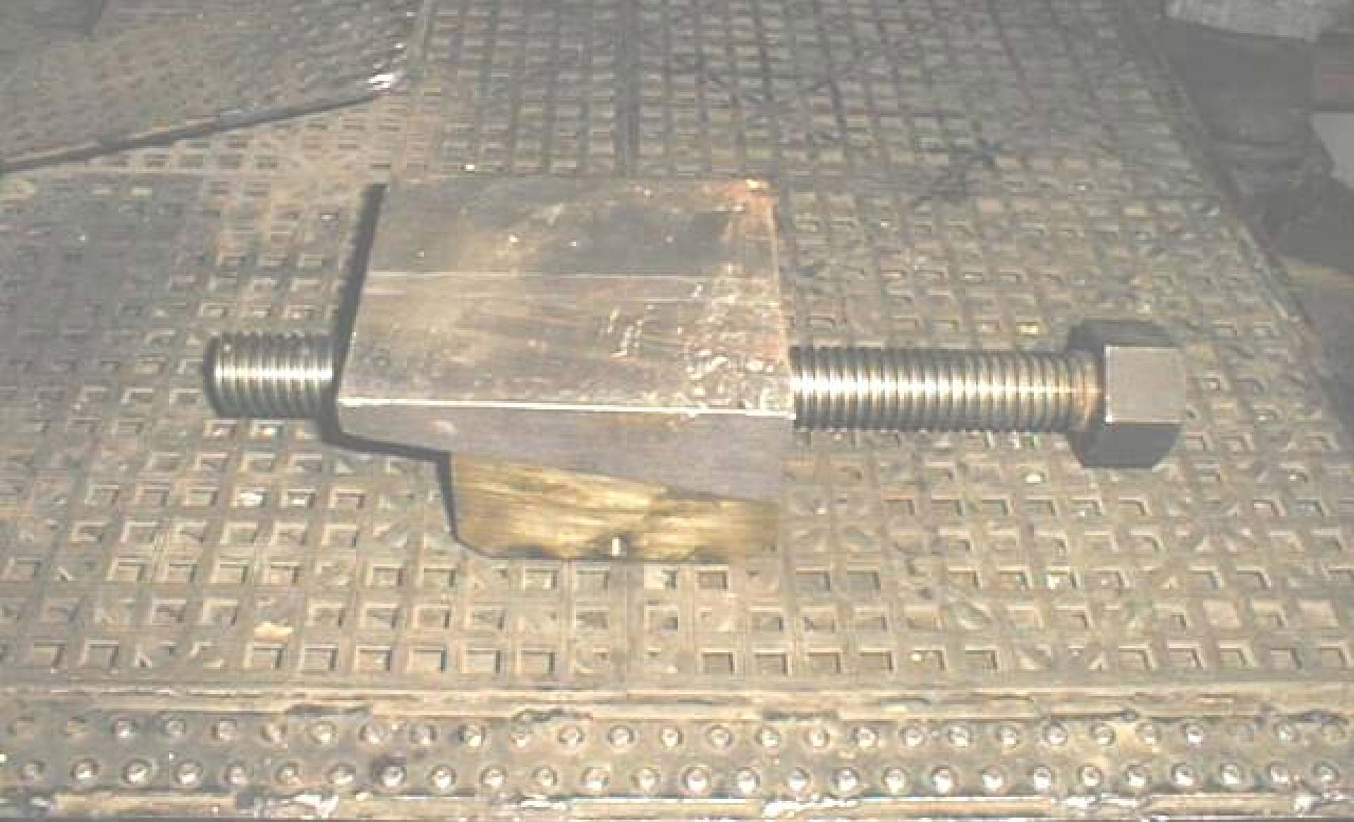
Wedges must be greased. If wedges are not tight the vibro will not put energy into the casing.
