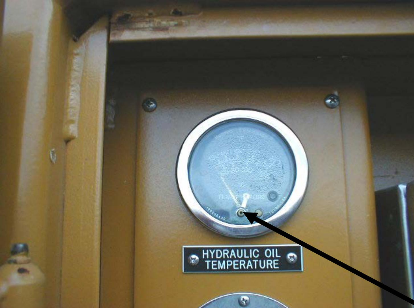
Hydraulic oil temp gauge and switch. Switch shuts engine down when oil temp passes setting. Set the maximum temp using a small allen wrench. Usually set at about 190 degrees.
